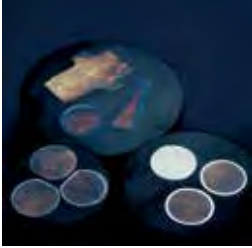
Crosscuts to check hardening depth.
