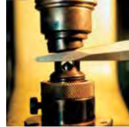
Special tool control for blade hardness.
