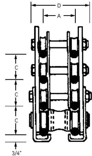
**Warning:** Safe working load displayed can only be achieved by utilizing Dayton Superior B12 High Strength Coil Rod and B25 Heavy Coil Nuts.
