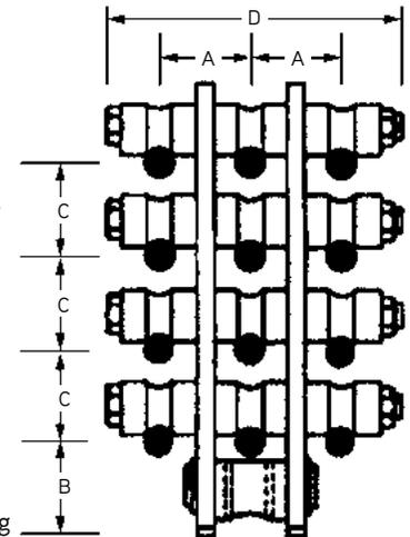
**Warning:** Safe working load displayed can only be achieved by utilizing Dayton Superior B12 High Strength Coil Rod and B25 Heavy Coil Nuts.
