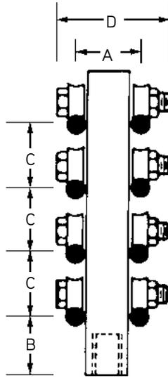
**Warning:** Safe working load displayed can only be achieved by utilizing Dayton Superior B12 High Strength Coil Rod and B25 Heavy Coil Nuts.
