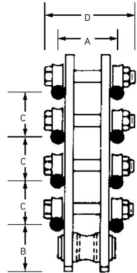
**Warning:** Safe working load displayed can only be achieved by utilizing Dayton Superior B12 High Strength Coil Rod and B25 Heavy Coil Nuts.
