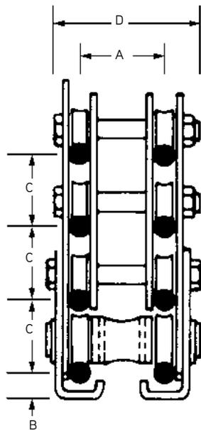
**Warning:** Safe working load displayed can only be achieved by utilizing Dayton Superior B12 High Strength Coil Rod and B25 Heavy Coil Nuts.
