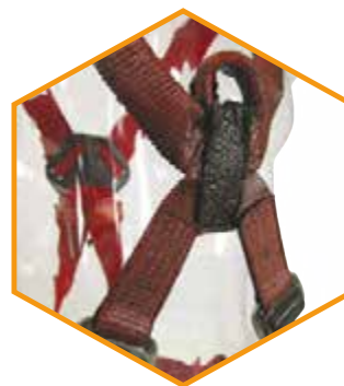
NYLON HARNESS EXPOSED TO ARC FLASH
